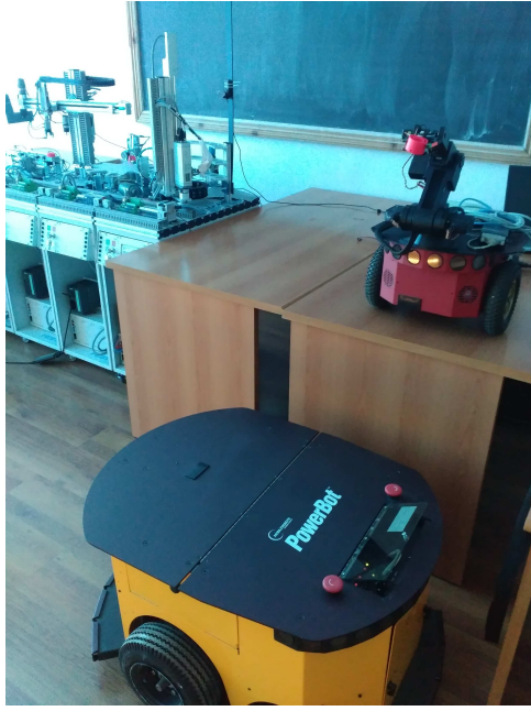
Fig. 8. The PowerBot mobile platform used in the real experimental scenario
